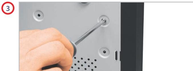
Screw through the holes in the base of the NVR or hard drive shelf, and into the four fixing holes in the bottom of the hard drive. (Screws supplied with hard drive.)
