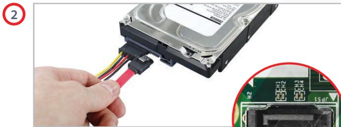
Now connect the SATA cable to the SATA socket on the hard drive. Connect the other end to the SATA socket on the PCB then place the drive in the NVR case.
