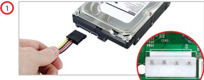
Connect the power cable to the power socket on the hard drive. Connect the other end (White plug) to the power socket on the PCB.
